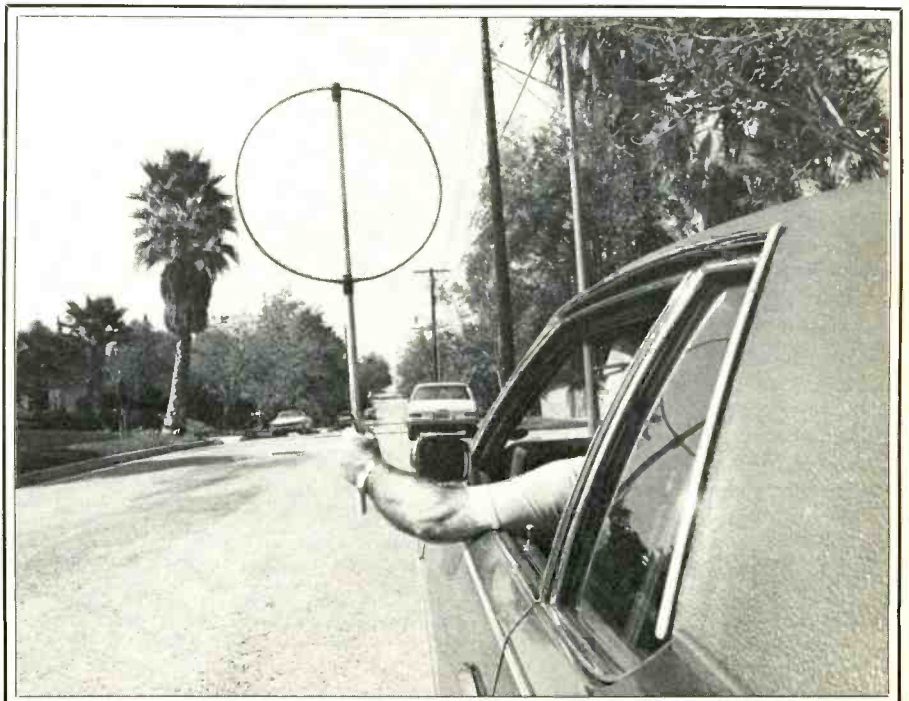
Signals from a "wire" are picked up and recorded on equipment in an unmarked vehicle within range of the low-power transmitter.
