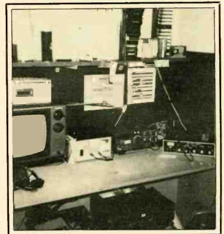
Renard's CW signals emanate from a Kenwood TS-130 transceiver via an MFJ antenna tuner.
